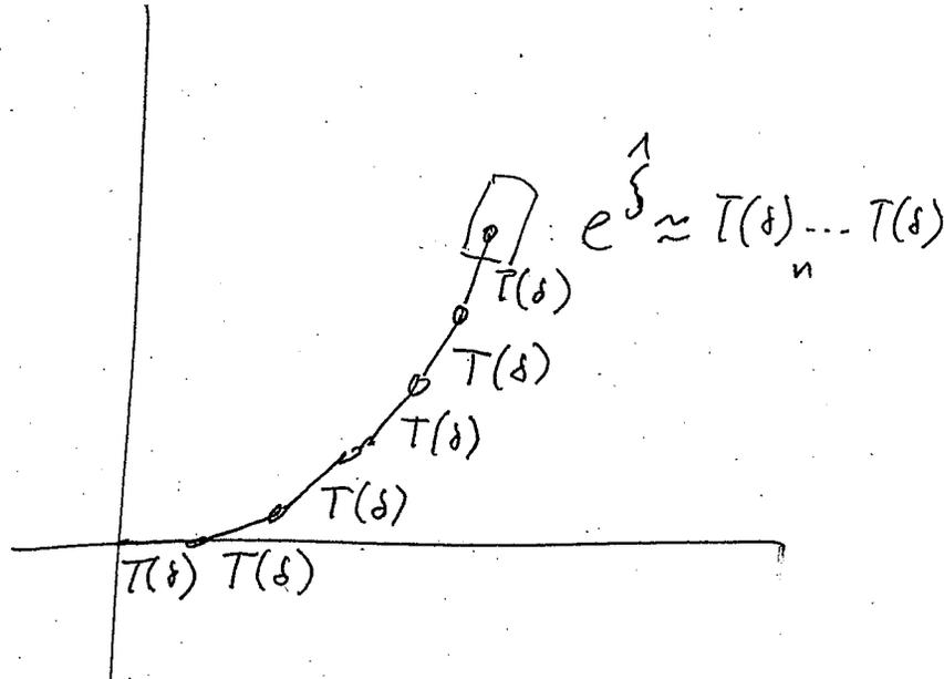
Figure 2: Approximating a circular trajectory with  $n$  steps.
