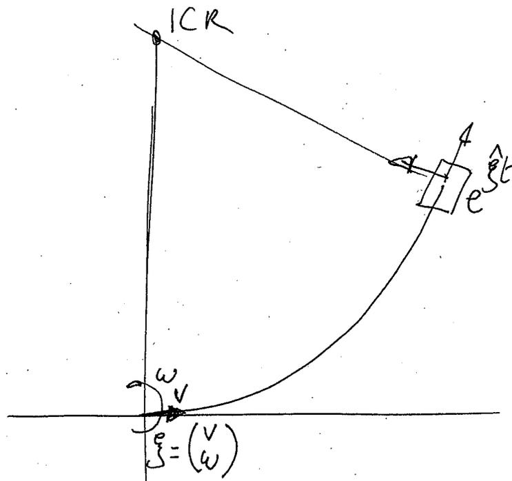
Figure 1: Robot moving along a circular trajectory.
